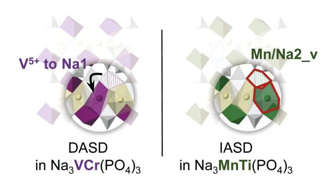
Illustration demonstrating the intrinsic anti-site defect (IASD) and the derivative anti-site defect (DASD) in polyionic compounds in sodium-ion batteries. Credit: Zhao Junmei
