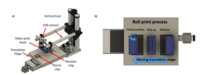
(a) Schematic representation of the roll printing setup. (b) Printing process (left to right), devices are released from a donor onto the roller print head and then released onto a receiver chip. Credit: *Optical Materials Express* (2023). DOI: 10.1364/OME.483657
